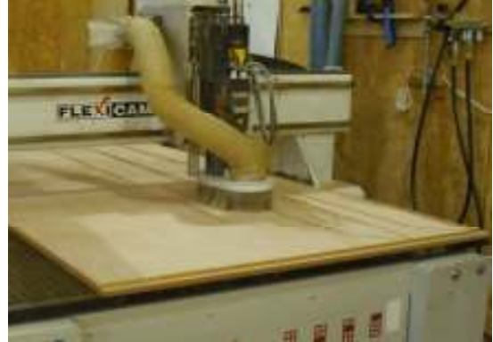
CNC machined and scarfed planks
